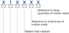
Convective heat resistance Contact heat resistance Burning behaviour
